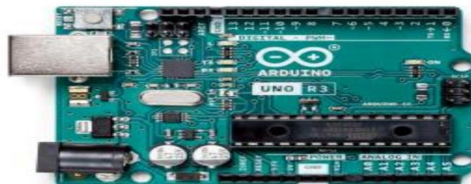
Figure 6: Arduino Uno board [35]
