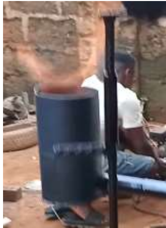
Figure 9b: Flaring of Syngas in a Burner without Expansion Drum but with Filtration Unit
