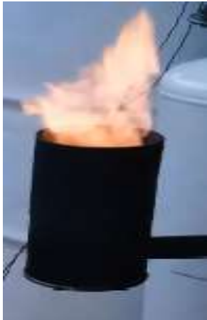
Figure 9a: Flaring of Syngas in a Burner without Expansion Drum and Filtration Unit
