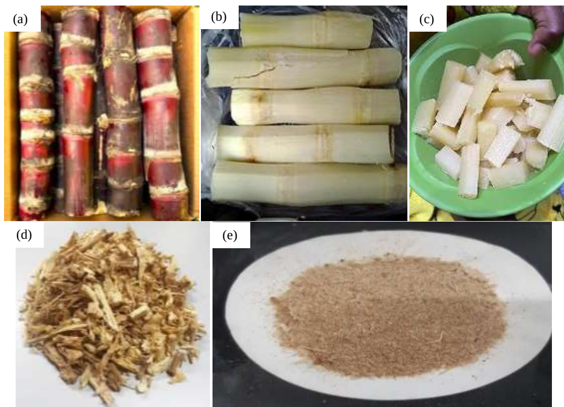
Figure 1: Steps implemented in processing SB: (a) as received stalks, (b) peeled, and (c) cut sugarcane before extracting the wet contents. (d) dried and charred bagasse, and (f) Pulverized bagasse.
