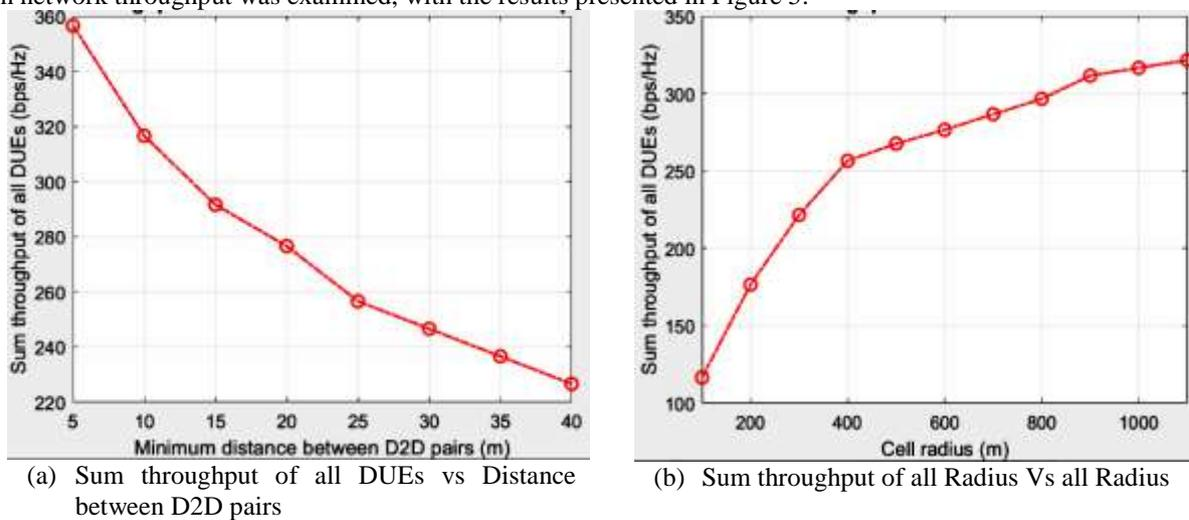
Figure 5: Distance and radius effect on throughput
