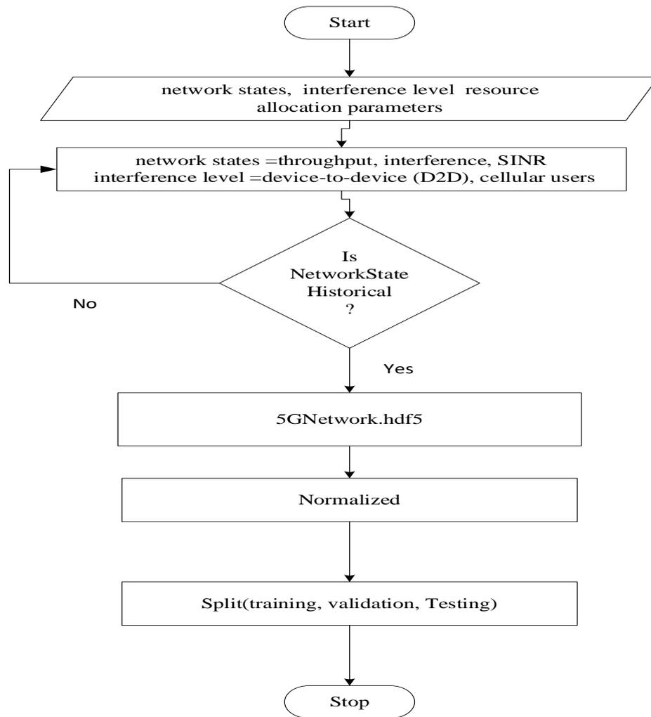
Figure 1: 5GNetwork.hdf5 flowchart
