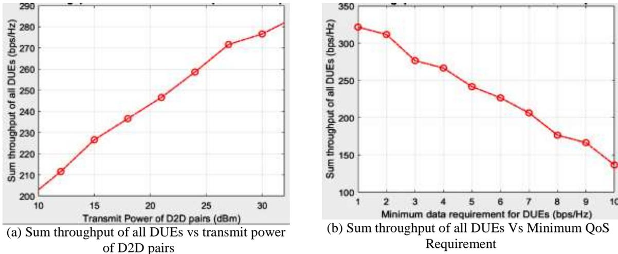
Figure 6: Transmit power and minimum QoS
