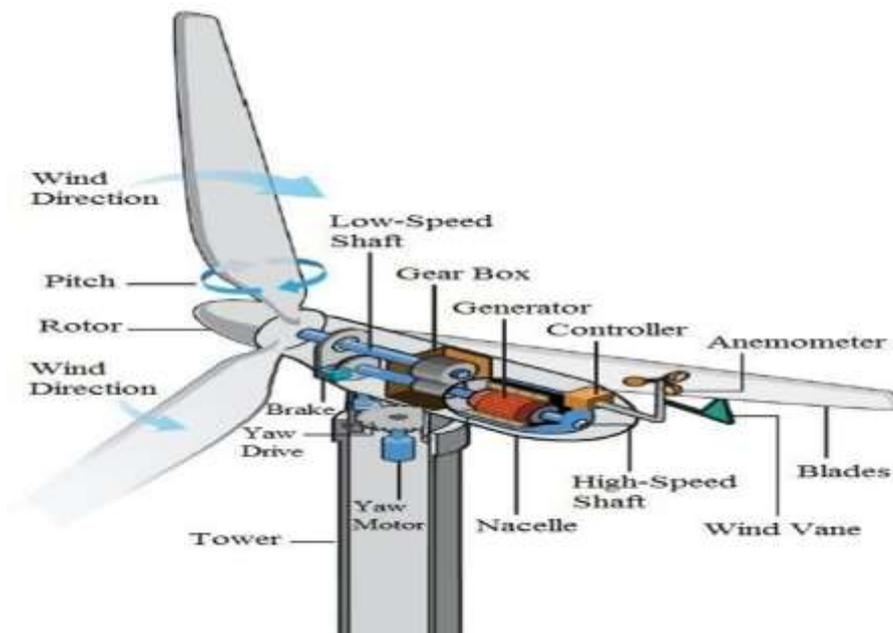
Figure 5: Horizontal Axis wind turbine (HAWT) [20]
