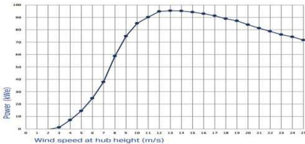
Figure 7: Power curve of a wind turbine [26]
