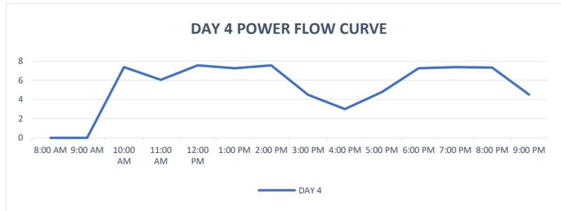
Figure 15: Graph of wind turbine power output against time for day 4
