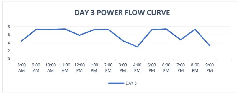
Figure 14: Graph of wind turbine power output against time for day 3
