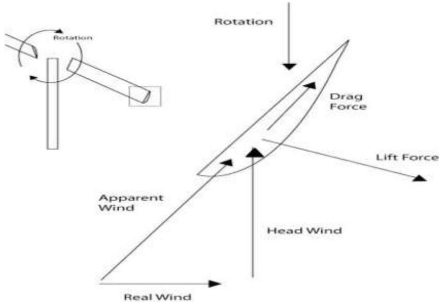
Figure 8: Lift/Drag forces experienced by turbine blades [27]
