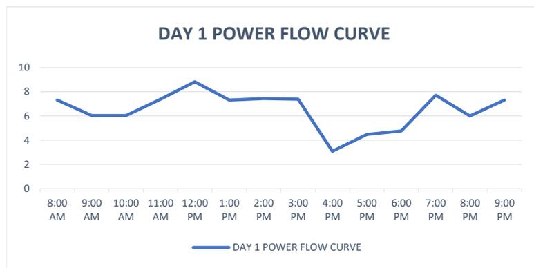
Figure 12: Graph of wind turbine power output against time for day 1
