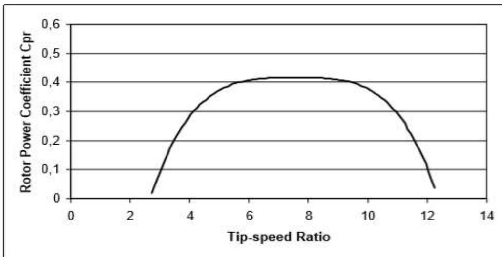
Figure 9: Power flow curve vs blade tip speed/wind speed [31]
