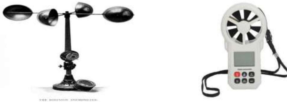
Figure 10: A cup and a hand-held anemometer [33]
