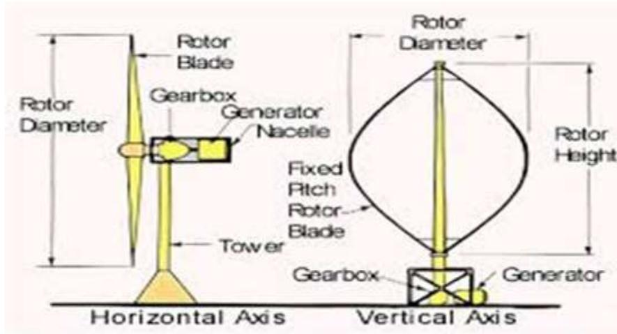
Figure 4: Horizontal and vertical wind turbine [20]
