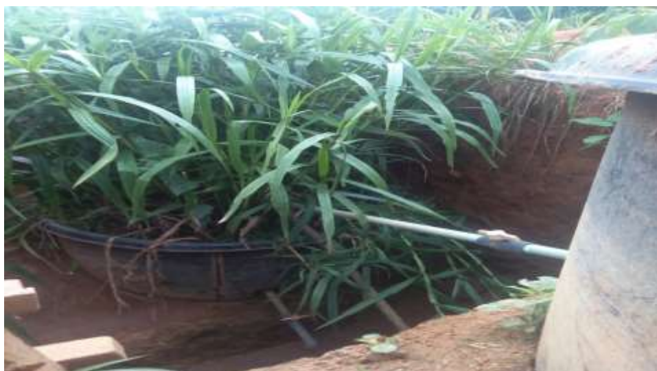
Figure 3: Constructed wetland planted with common reed at the experimental field
