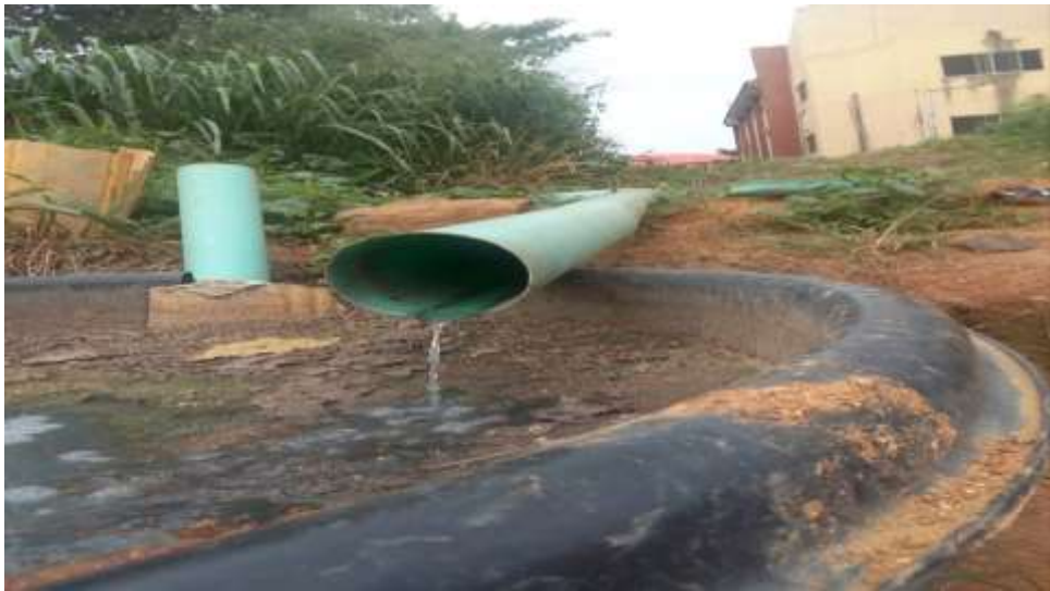
Figure 2: Raw greywater coming from the hostel to the sedimentation tank at the experimental field
